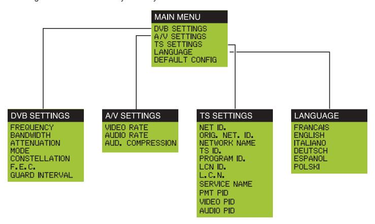
In order to go from one menu to the other use the move up/down ( $\triangleleft$  and  $\triangleright$ ) keys to select the menu options. Press the enter ( $\checkmark$ ) button to select this option. Press the cancel (X) button to go back to the previous menu.
